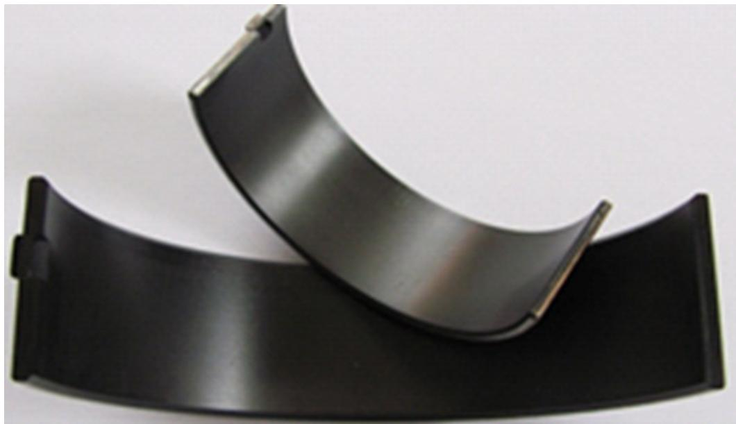
The new material has been tested in comparison with traditional tri-metal bearings. The results of the comparative tests conducted in King's Test Rig are presented in figure below. The tests were performed under a bearing load of 10,200 psi for 4,300,000 cycles. Both conventional and pMax Black™ bearings had the same dimensions.
